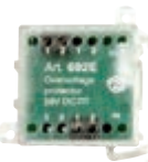
692E Overvoltage protection device
